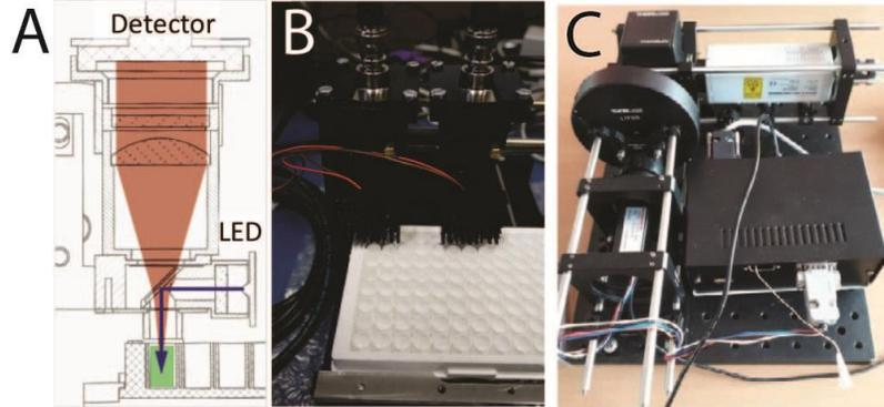
Fig. 1. (A) Schematic of the ELISA plate compatible sensor head. (B) Photo of the ELISA plate compatible instrument. (C) Photo of the cuvette based instrument.
